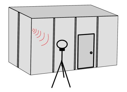
test process faces a challenge. Most environments are saturated with RF energy from broadcast radio, television, cellular, Wi-Fi, satellite transmissions, solar activity, and many other sources. Shielded enclosures isolate the test process from outside signal interference and enable engineers to more accurately measure device signal levels and attenuation for comparison to regulations.
