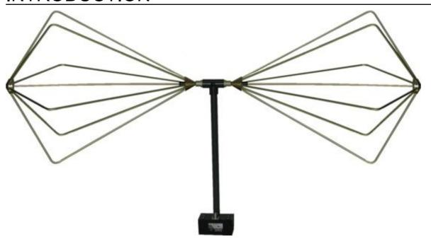
The SAS-544 Biconical Antenna is designed with a coaxial wound balun for increased power capability and intended for both transmitting and receiving high electromagnetic RF fields. This Biconical antenna may be used for radiating immunity measurements. Whether testing in a shielded enclosure, or outdoors, the rugged construction of the A.H. Systems Biconical antenna will ensure long life, and reliable performance.
