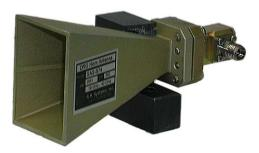
The SAS-574 Double Ridge Guide Horn Antenna is a broadband antenna that offers excellent performance over the frequency range of 18 GHz to 40 GHz. The original design was to have a 30-degree beamwidth, which is ideal for EMI measurements and compliance testing.
