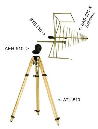
Mount the antenna such that the elements are parallel to the ground for horizontal polarization testing, or perpendicular to the ground for vertical testing. The horizontal beamwidth of the Bilogical is approximately 45 degrees and it should be pointed or aimed in the direction that the received signal is coming from.
