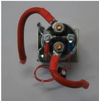
Uninstalled 100 A relay
