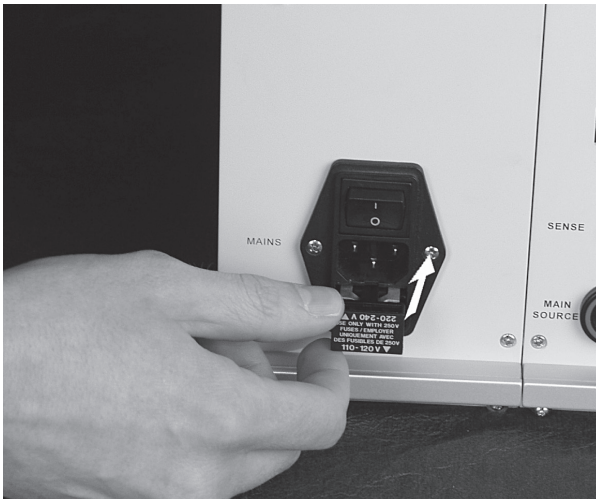
Picture 4-7: Fix the drawer to the input connector assembly.
