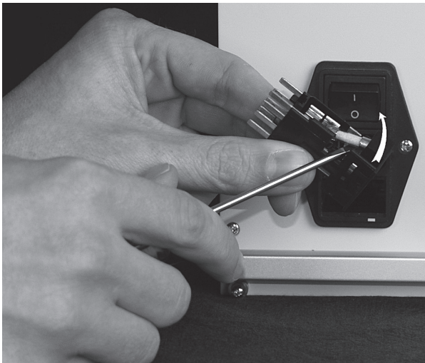
Picture 4-5: Remove defect fuses.
