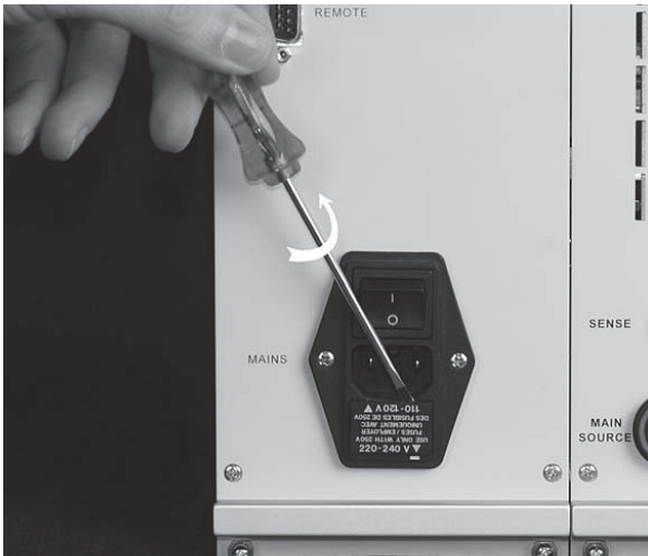
Picture 2-2: Loosen the drawer using a screwdriver
