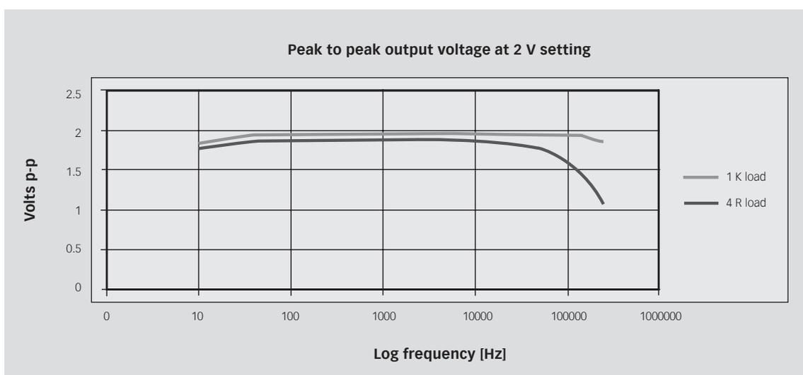
Picture 6-14: Output voltage vs frequency for a voltage setting of 2 V<sub>pk-pk</sub> at 1 k $\Omega$  and 4  $\Omega$  loads
