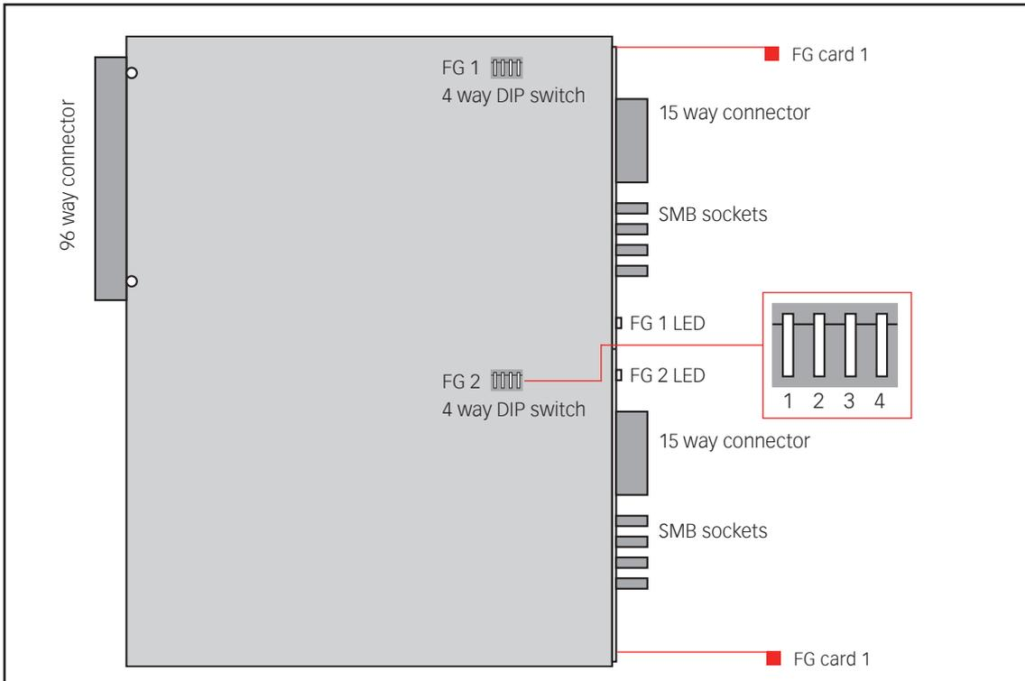
**Picture 3-13: FG 5620 solder view showing the 4 way DIP switch**
