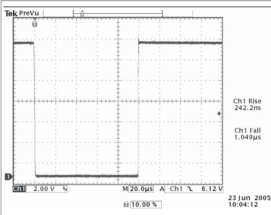
Picture 6-8: 13.5 V Dropout into 1 kΩ load for 100 μs
