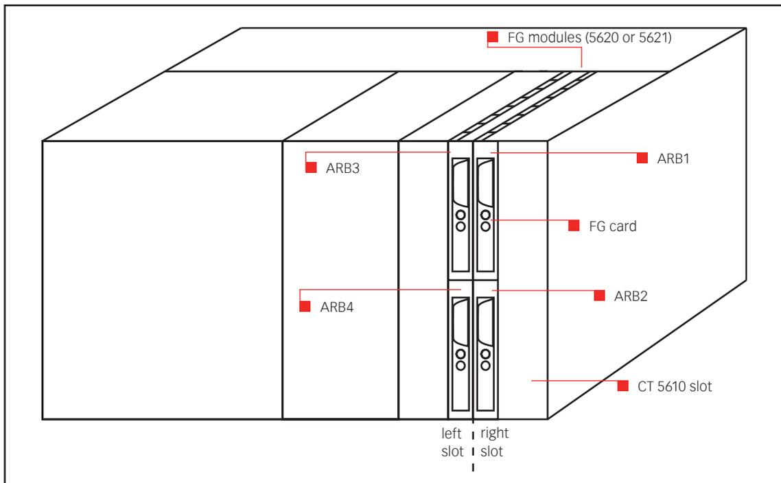
Picture 3-17: Basic chassis containing 2 FG 5621 (4 ARB cards) in left and right slots
