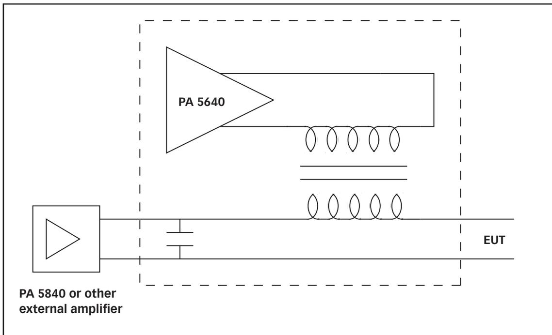
Picture 4-2: Conducted sine waves from the NSG 5602
