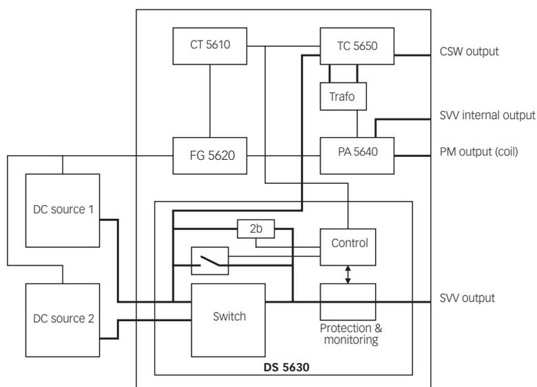
Picture 2-2: Functional block diagram of the NSG 5600 system
