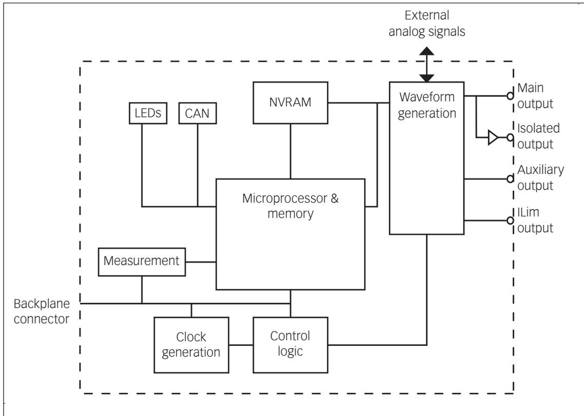
**Picture 4-8: FG 5620 Module functional block diagram**
