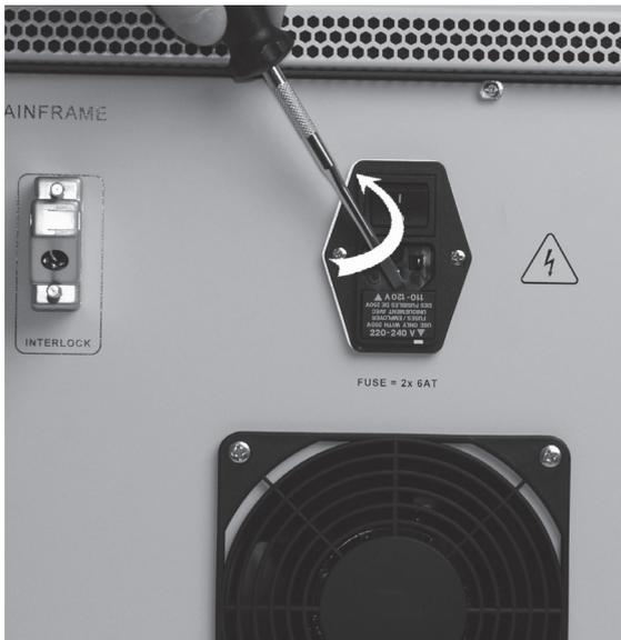
**Picture 3-2: Loosen the drawer using a screwdriver**
