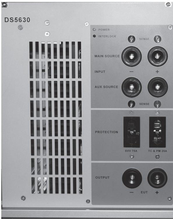
Picture 4-12: DS 5630 Front panel connectors
