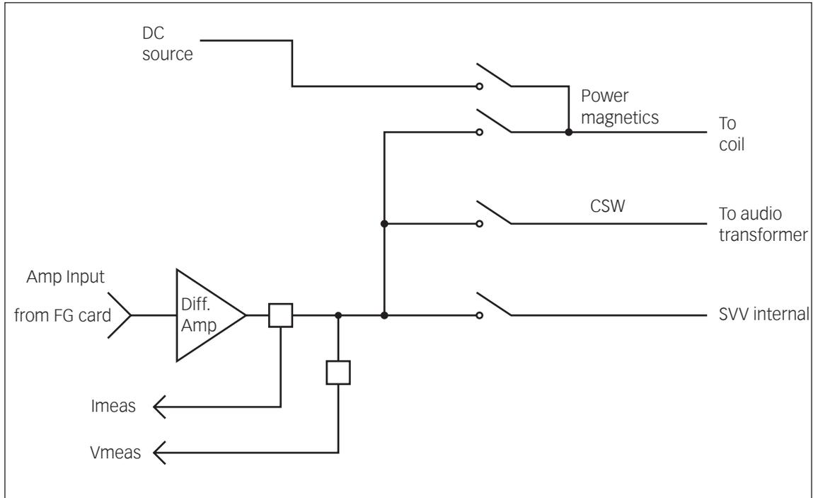
**Picture 4-14: Basic block diagram of the PA 5640**
