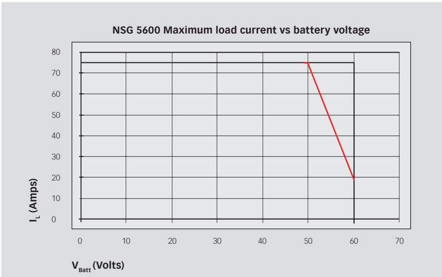
Picture 6-5: Pulse 4d safe operating area (load current vs battery voltage)
