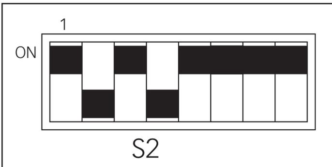
**Picture 3-10: Switch S2 - CAN address**
