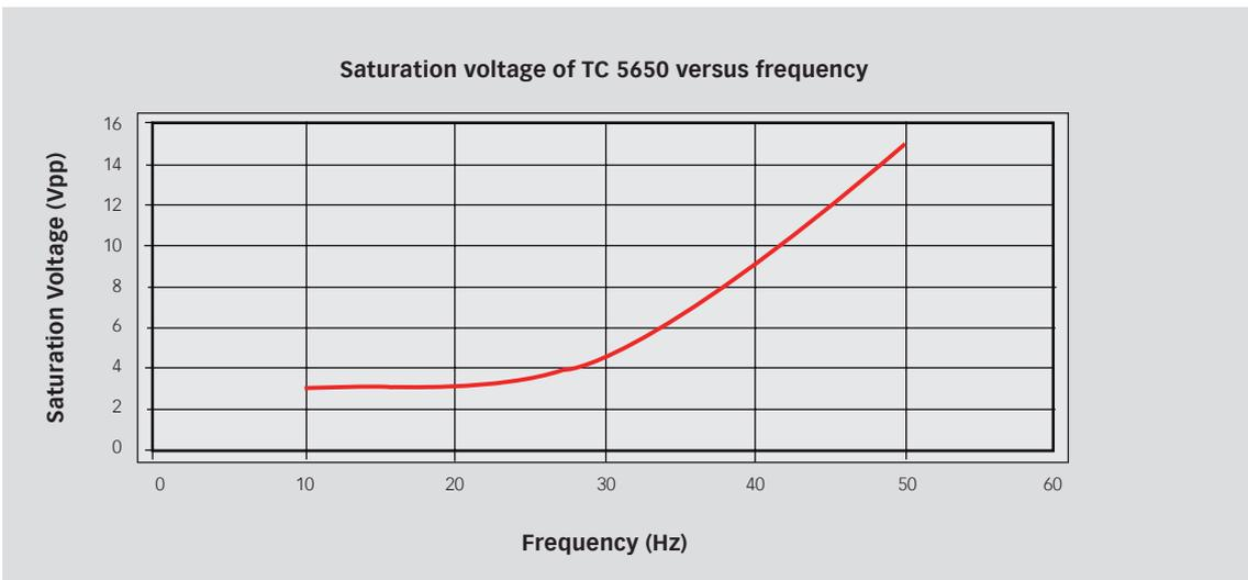
Picture 6-16: TC 5650 Transformer saturation voltage vs frequency
