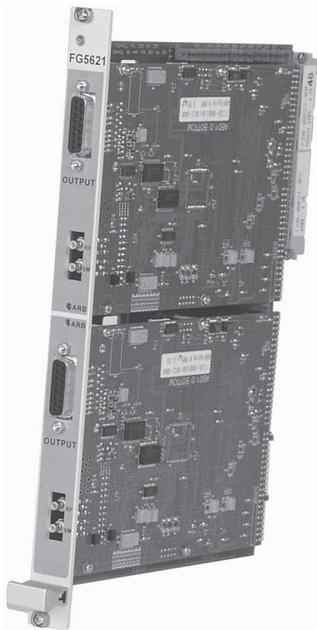
Picture 4-7: FG 5620 Function generator module for arbitrary waveforms
