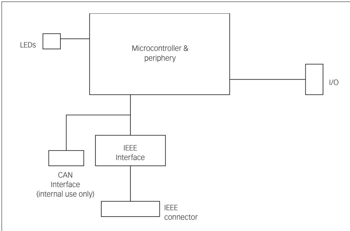
**Picture 4-5: CT 5610 Controller module functional block diagram**
