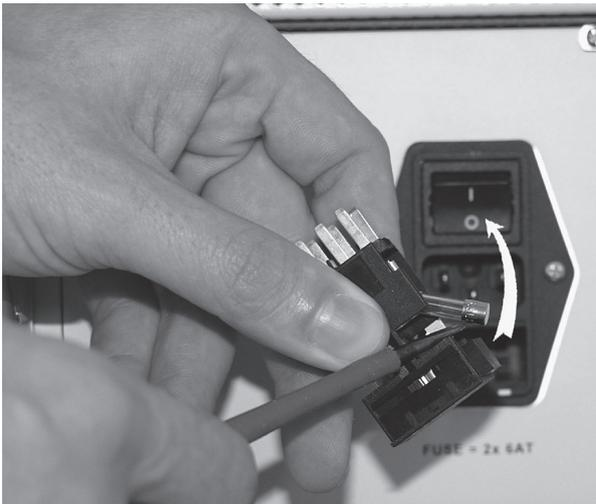
**Picture 4-5: Remove defect fuses**
