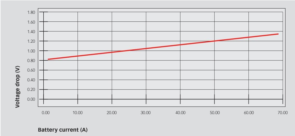
Picture 6-4: Pulse 4d Battery voltage drop vs battery current
