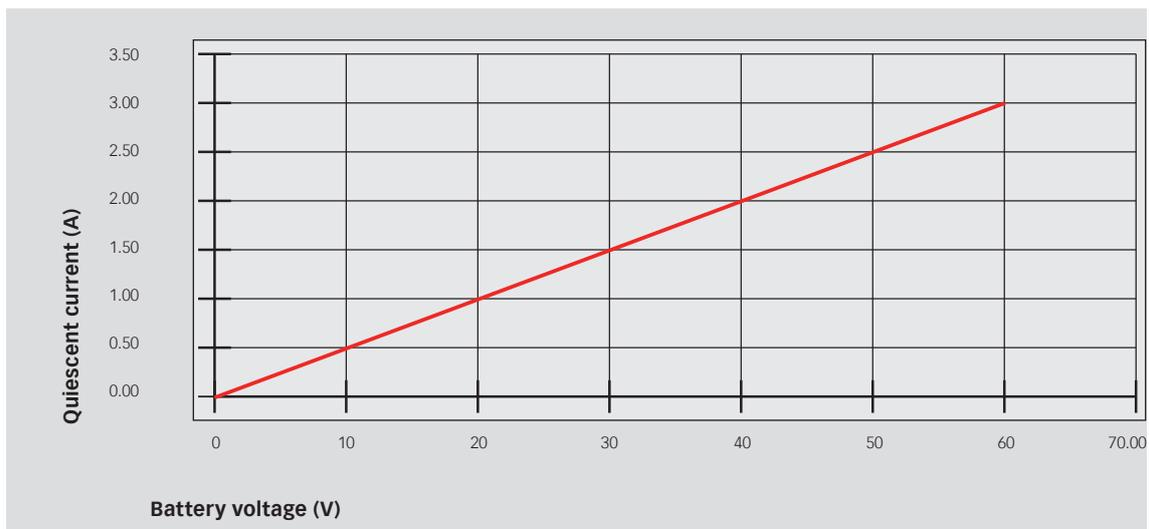
Picture 6-6: Pulse 4d quiescent current vs battery voltage
