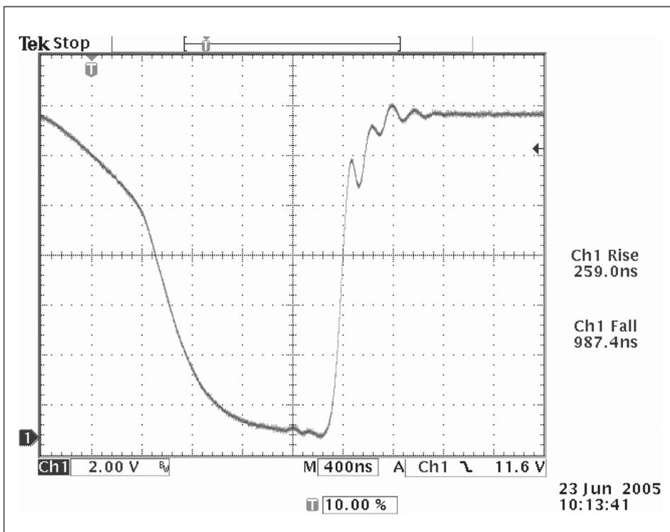
Picture 6-10: 13.5 V Dropout into 1 k $\Omega$  load for 3  $\mu$ s
