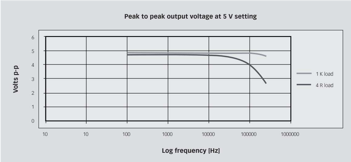
Picture 6-15: Output voltage vs frequency for a voltage setting of 5 Vpk-pk at 1 kΩ and 4 Ω loads
