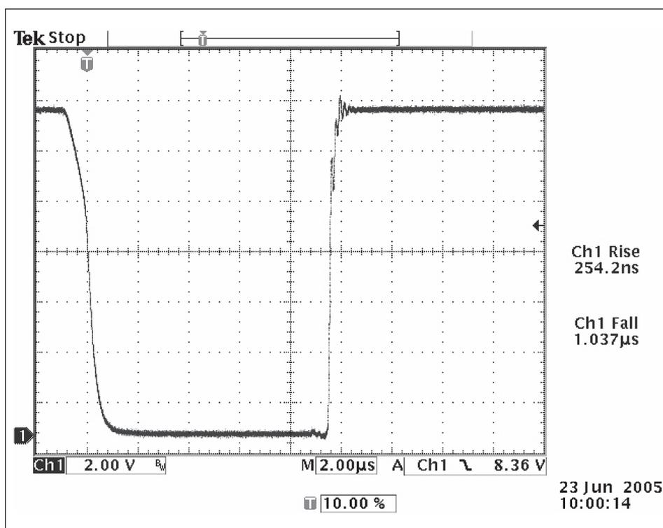
Picture 6-7: 13.5 V Dropout into 1 kΩ load for 10 μs
