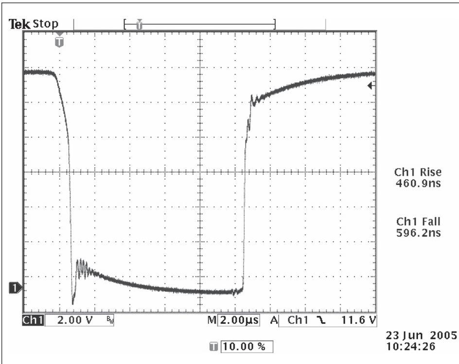
Picture 6-9: 13.5 V Dropout into 1 Ω load for 10 μs
