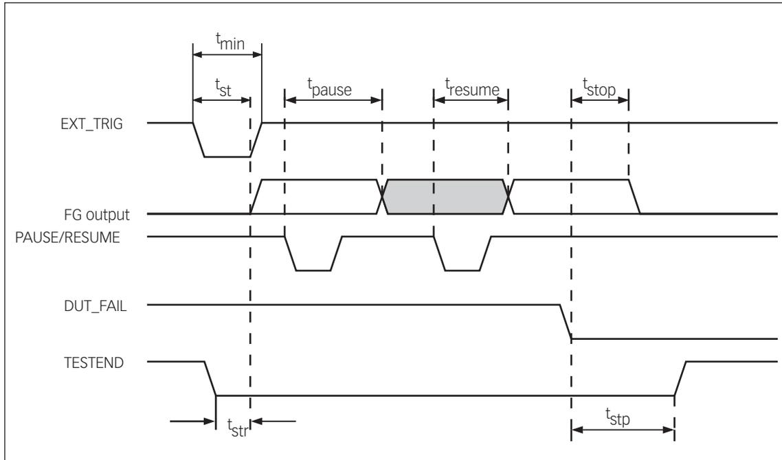
Picture 6-1: Auxiliary signals timing diagram
