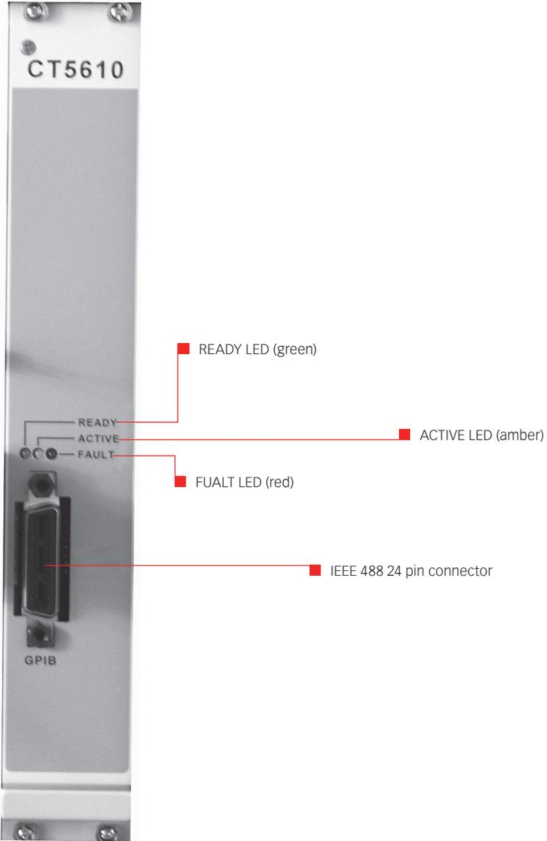
Picture 4-6: CT 5610 Module front panel connector
