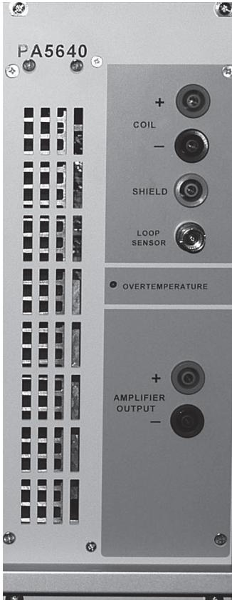
Picture 4-16: PA 5640 Front panel connectors
