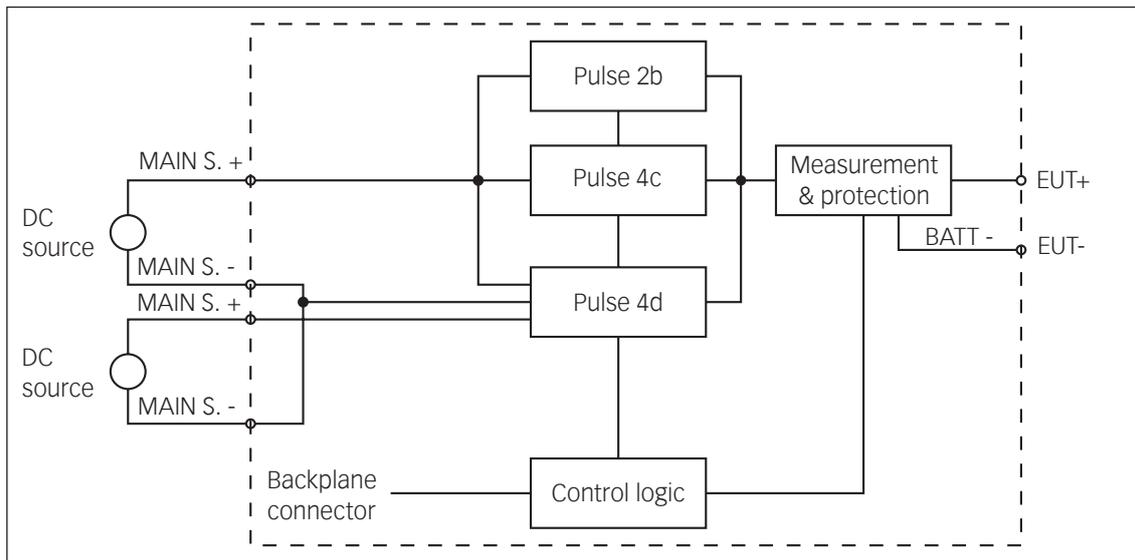
**Picture 4-11: Block diagram of DS 5630 showing 2 external sources connected to it for pulse 4d**
