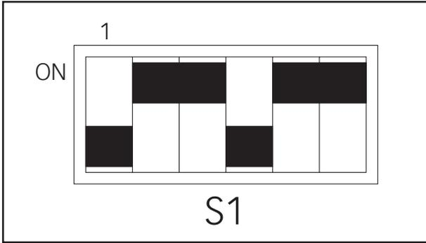
**Picture 3-9: Switch S1 - GPIB address**
