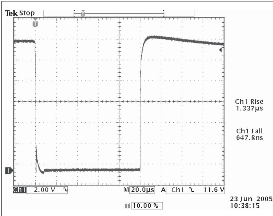
Picture 6-12: 13.5 V Dropout into 1  $\Omega$  load for 100  $\mu$ s
