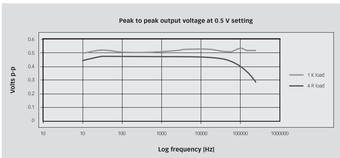
Picture 6-13: Output voltage vs frequency for a voltage setting of 0.5 V<sub>pk-pk</sub> at 1 k $\Omega$  and 4  $\Omega$  loads
