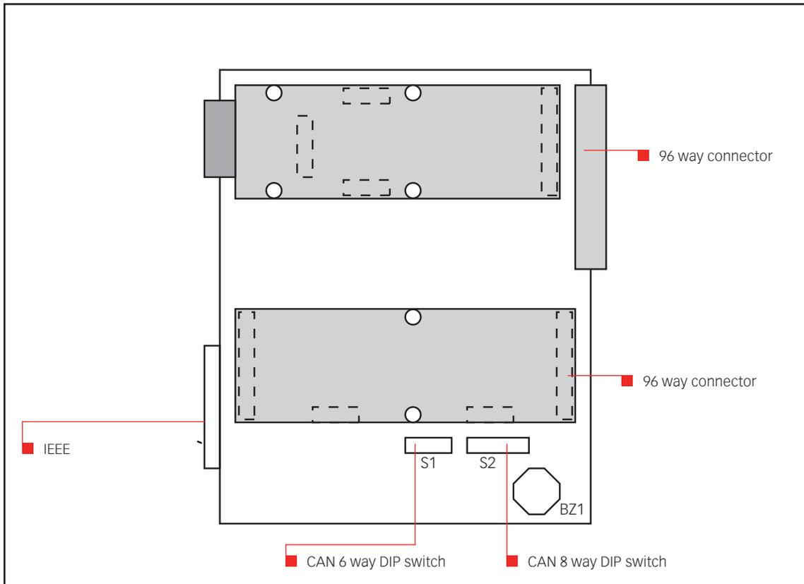
**Picture 3-8: CT 5610 Module top view with DIP switches S1 and S2**
