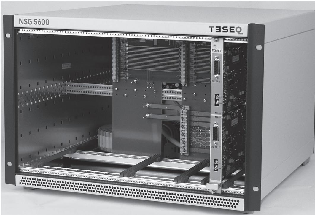
Picture 3-17: Basic chassis containing 2 FG 5621 (4 ARB cards) in left and right slots.
