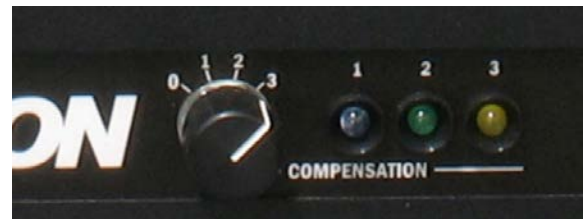
Figure 3.3 Amplifier Compensation Control
