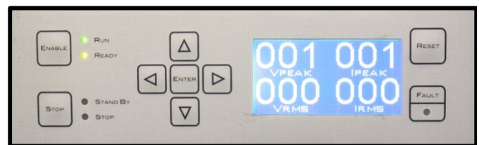
Figure 3.10 Enabled Amplifier LED Display
