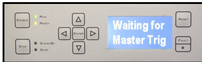
Figure 4.2 Slave Amplifier Bi-Level Setting at "Waiting for Master Trigger"
