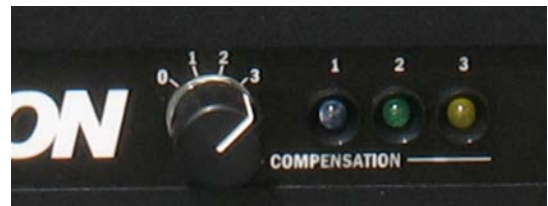
Figure 10.3 4301 amplifier module compensation control and indicators
