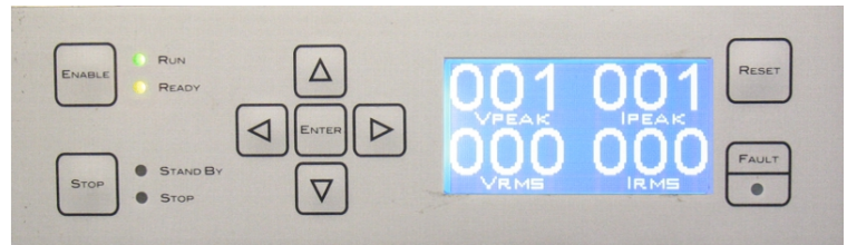
Figure 10.2 4301 amplifier module control panel
