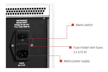
To insert a fuse, pull the fuse-holder out of the connector, insert 2 fuse cartridges  $2 \times 3.15$  AT (slow blow) into the holder and put the holder back.
