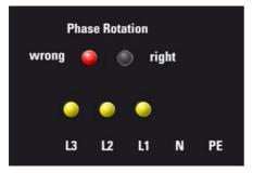
Not all EUT power lines provide power and the phase rotation is wrong too. All phase of the EUT in power need to be checked and re-plugged.
