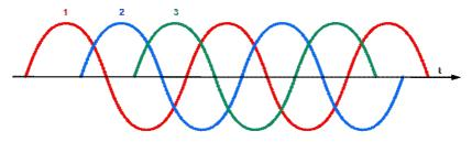
However, if we reverse the rotation winding 2's waveform will be leading 120° ahead of 1 instead of lagging, so the coupling point of a synchronous coupling will be wrong, since the zero crossing of L1 is measured and calculated for the other lines. The counter clockwise rotation phase sequence is 2-1-3, which is wrong.
