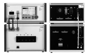
If a NSG 3040 goes with a CDN 3063 then the 3-phase coupler is default and active in the meaning that surge and EFT pulse will be coupled into the CDN 3063, while the PQT test is available at the NSG 3040 EUT output. Performing PQT test can realized without disconnecting or switching of the CDN 3063 (internal CDN of NSG 3040 is called CDN 3041).
