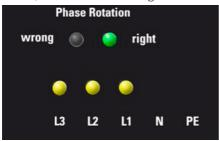
The EUT power lines provide all power, but the phase rotation is wrong. In this case the exchange of line L1, L2, or L3 will solve the rotation problem.
