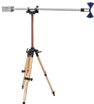
VSQ 3002, assembled for the frequency range 800 to 3000 MHz
