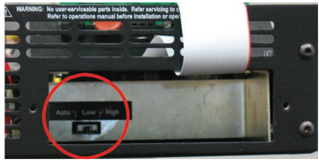
Figure 4.14 – Bi-Level Power Switch Location
