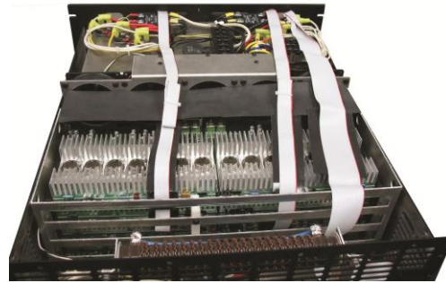
Figure 7.2 - Amplifier Cover removed for inspection
