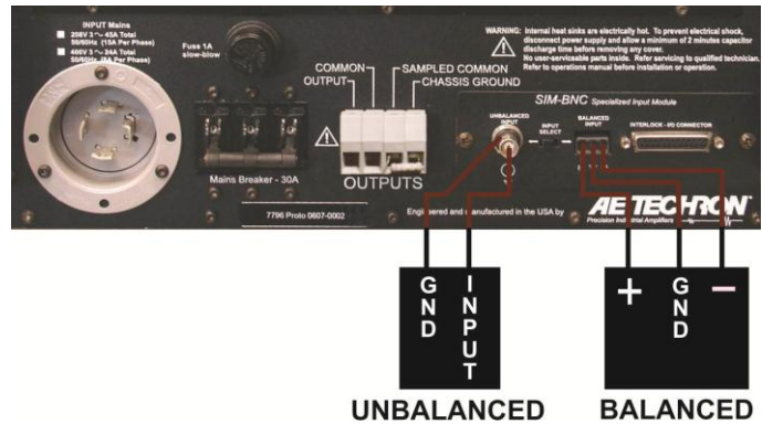
Figure 2.6 – Wiring for Unbalanced or Balanced Input Connector
