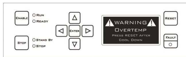
Figure 3.15 - Over-Temperature Fault LCD Display
