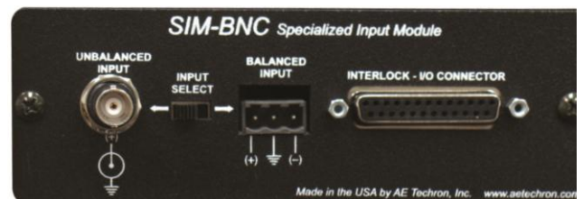
Figure 2.5 – Specialized Input Module (“SIM”) card
