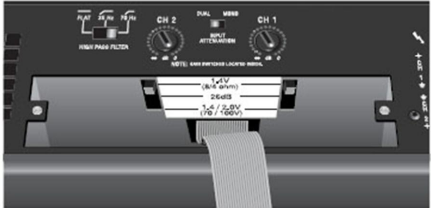
Figure 4.1 – Input Sensitivity Switches Location
