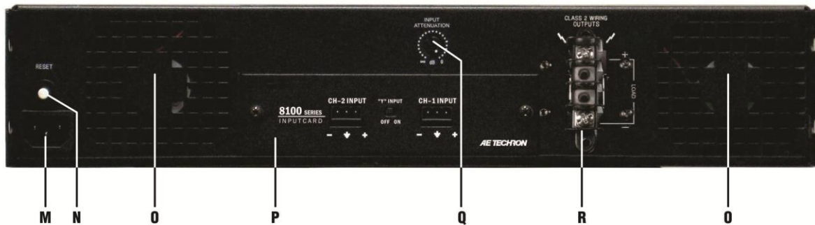
Figure 3.2 – 8102 Back-Panel Controls and Connectors
