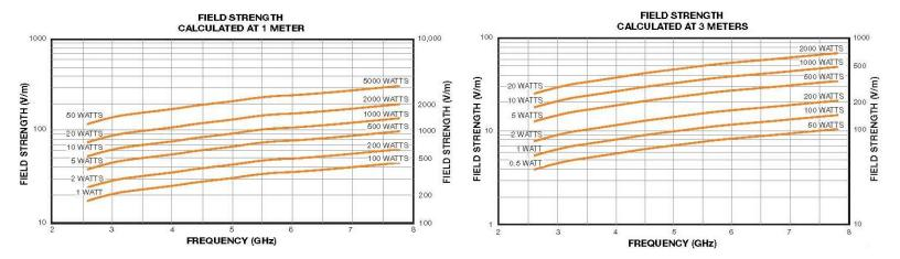
Field strengths have been measured in free-space conditions. Individual shielded rooms, amplifiers, and test-system conditions will influence performance. Field strength also varies with frequency and position of antenna and EUT in non-anechoic testing environments.
