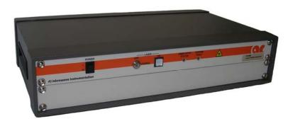
The FI7000 interface provides both power to and communication with the FL/PL 7000 series probes. A low-level loop back fiber optic connection is used to sense unexpected disconnect of laser driven fibers to ensure user-safe operation. As an additional safety measure, shuttered connectors are used on all fiber optic connections to and from the probe.
