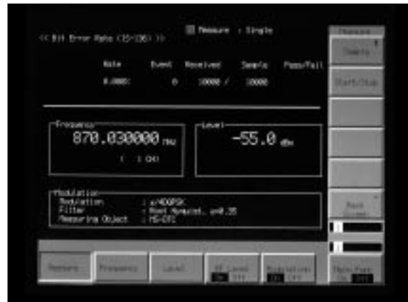
Bit error rate measurement (IS-136A)
