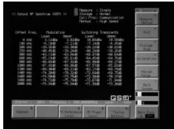
Output RF spectrum measurement (GSM)
