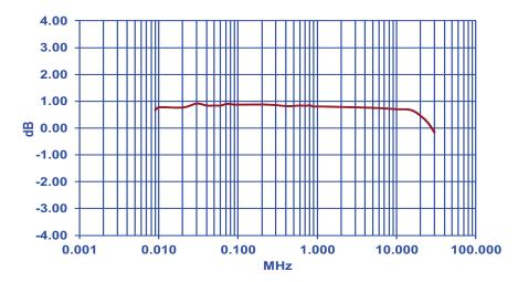
Field strength (dBuV/m) = Output measured(dBuV) + Antenna factor(dB)
