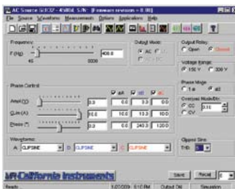
Soft front panel control through Windows GUI.
