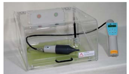
ESD3000 with remote DM for testing explosive devices
