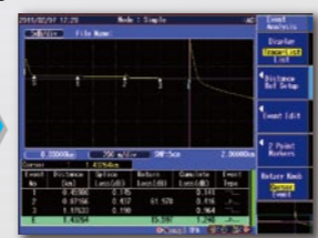
Waveform analysis screen of OTDR function
