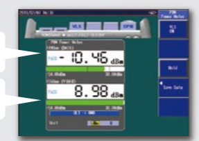
PON optical powermeter screen
