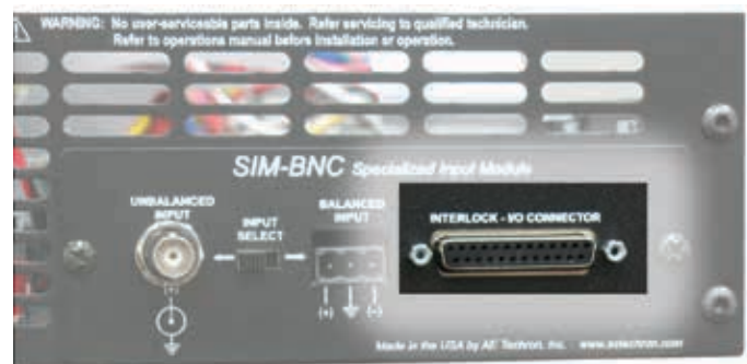
Figure 9.3 – Interlock I/O Connector
