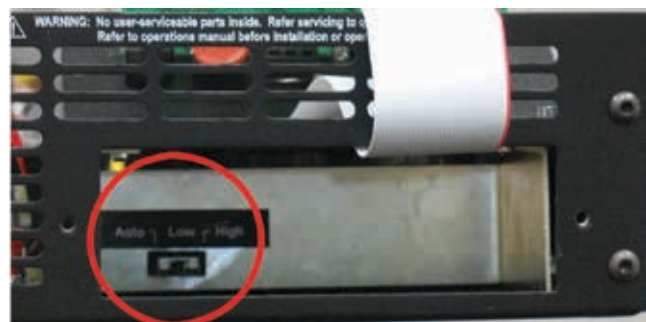
Figure 5.13 – Bi-Level Power Switch Location
