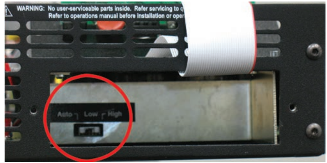
Figure 5.13 – Bi-Level Power Switch Location
