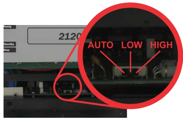
Figure 5.7 – Bi-Level Power Switch Location
