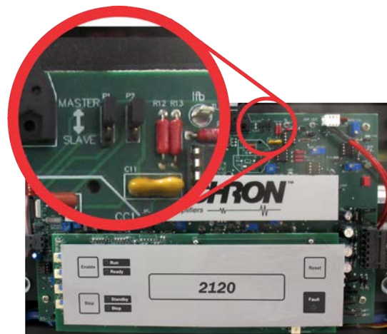
Figure 5.1 – Master or Slave Setting
