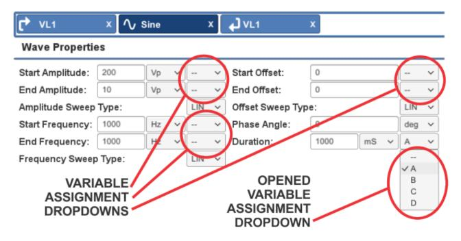
Find the waveform property to be varied within the loop, and then use the variable assignment drop-down to select a letter. After variable assignment, the input box for that property will be grayed to indicate its status as a variable. Check to make sure that the units being used for the property to be varied are the system default units (Vp for amplitude, Hz for frequency, VDC for offset, and ms for duration).
