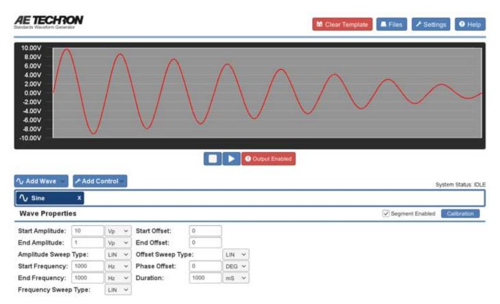
To add additional waveforms to the active test, select additional waveforms from the drop-down menu. New waveforms will be added sequentially and will appear to the right of the selected control or waveform in the active window.
