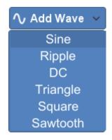
When you choose a waveform from the Add Wave drop-down menu, the default waveform of that type is added to the active window. Click on the tab or the waveform in the display to open the Properties form containing the available property settings for that waveform. See the individual entries in this Help system for more information about the settings available for each waveform type.
