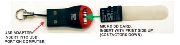
The microSD card contains the SWG Setup.exe file that is used to install the remote access SWG program on a Window's computer. For more information, see the topic *"3110 via Network."*
