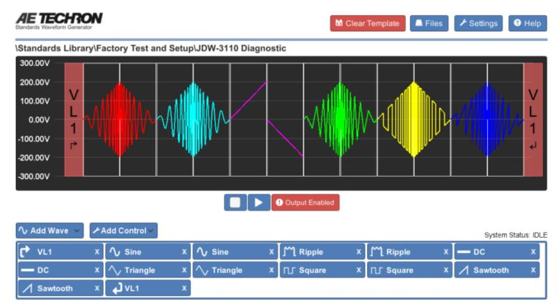
One or more waveforms and/or controls that have been added to the active test window can be run using the controls located below the SWG's active window.
