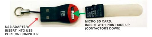
Remove the micro SD card from the USB adapter and insert the card into the card slot located on 3110 Controller back panel. Be careful when installing the card to insert the card with the printed side UP. The card must also be inserted in a straight line directly into the card slot. If the card is inserted at an angle, it may miss the internal card slot and be inaccessible from your 3110 unit.
