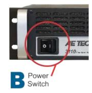
C. If the amplifier has a gain control, turn it fully ON (clockwise). Then turn the POWER switch ON to power up the amplifier.
