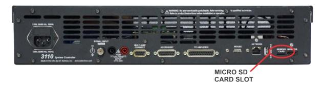
3. Turn on the 3110 Controller and allow the software interface to load. Then locate and press the Files button to open the Files explorer. Open the SDCARD directory and then locate the update Apk file you saved. NOTE: If the SDCARD directory won't open, the microSD card is not being recognized by the 3110 controller. Check the insertion of the microSD card. It may not have been inserted properly or completely.
