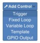
When you choose a control from the Add Control drop-down menu, an icon representing that control type is added to the active window, and a form containing the available settings for that control opens below the active test display. See the individual entries in this Help system for more information about the settings available for each control type.
