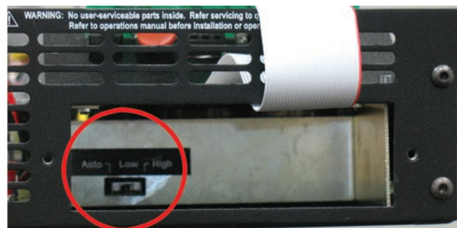
Figure 5.13 – Bi-Level Power Switch Location
