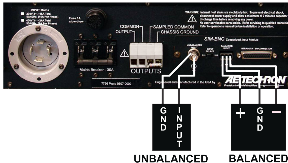
Figure 2.4 – Wiring for Unbalanced or Balanced Input Connector
