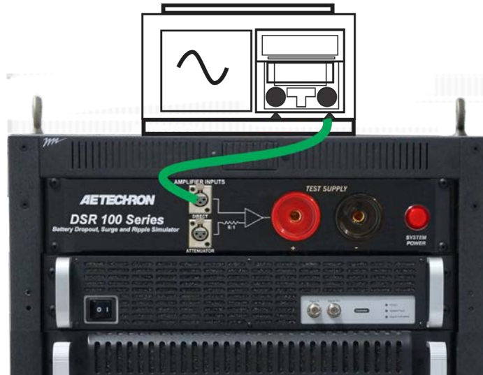
Figure 2.6 – Connecting a Stand-alone Signal Generator to the Direct Amplifier Input
