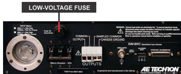
Figure 5.2 – Amplifier Module’s Low-voltage Fuse Location
