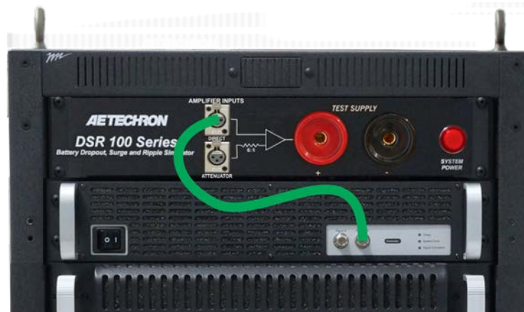
Figure 2.5 – Connecting the 3110 to the Direct Amplifier Input
