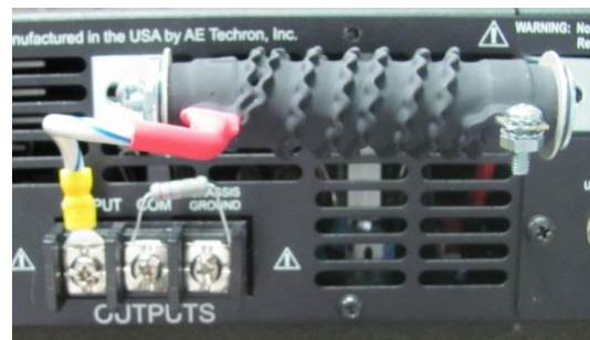
Figure 4.3 – 2105/7224 Ballast Resistor Connected to Output Terminal
