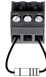
Figure 3.9 - Terminating the Amplifier Input
