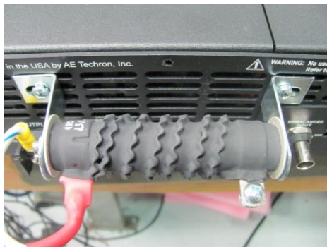
Figure 4.1 – 2105/7224 Ballast Resistor Mount
