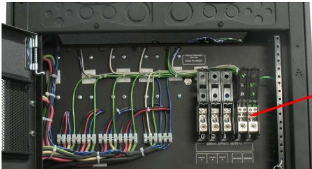
Figure 2.2 Barrier Strip Wiring Panel (4301-240, 4301-180, and 4301-120 systems)
