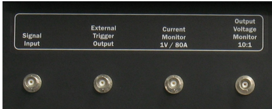
Figure 2.8 Signal Input, External Trigger Output, Current and Voltage Monitor BNC connectors (4301-240 model shown)
