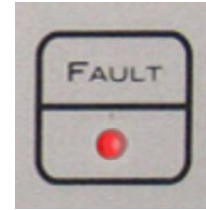
Figure 3.8 Fault Status Indicator
