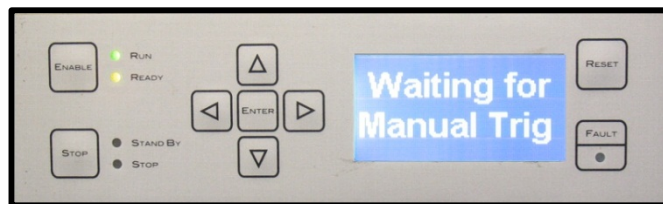
Figure 4.1 Master Amplifier Bi-Level Setting at "Waiting for Manual Trigger"
