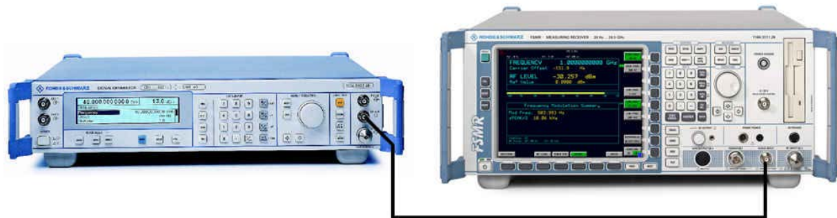
Fig.2-13 Audio measurement setup
