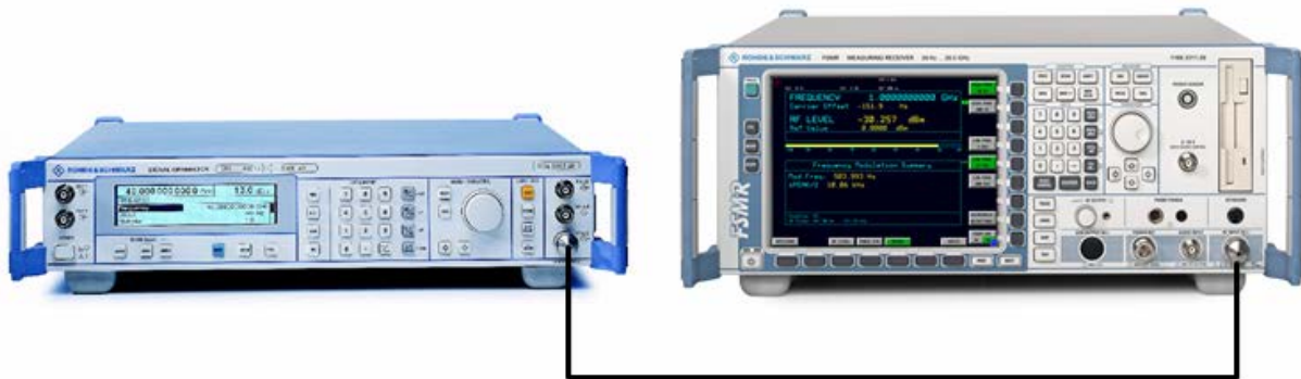
Fig.2-9 AM modulation measurement setup
