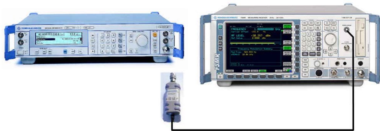
Fig.2-2 RF Power measurement setup
