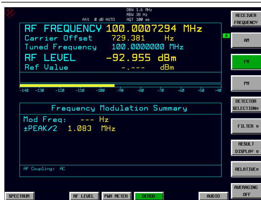
Fig.2-1 Display after selecting the default setup in receiver mode
