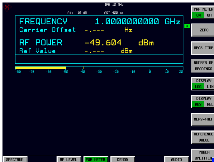
Fig.2-3 RF power measurement after Zeroing
