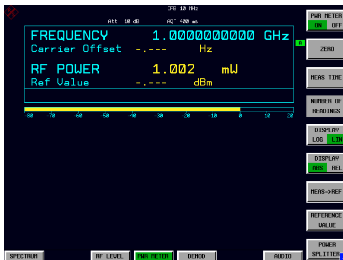
Fig.2-4 RF power measurement in UNIT Watt
