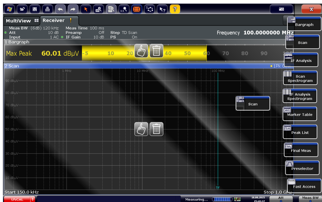
Figure 4-1: Moving a window in SmartGrid mode
