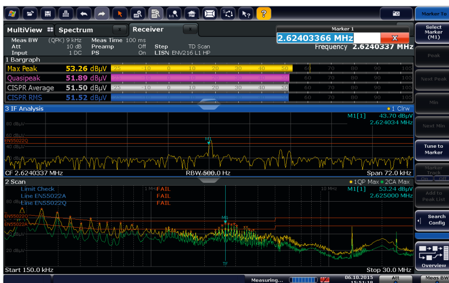
IF analysis (middle) and scanned RF spectrum (bottom).
