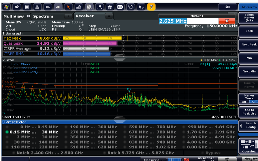
Display of trace and active preselection filter.
