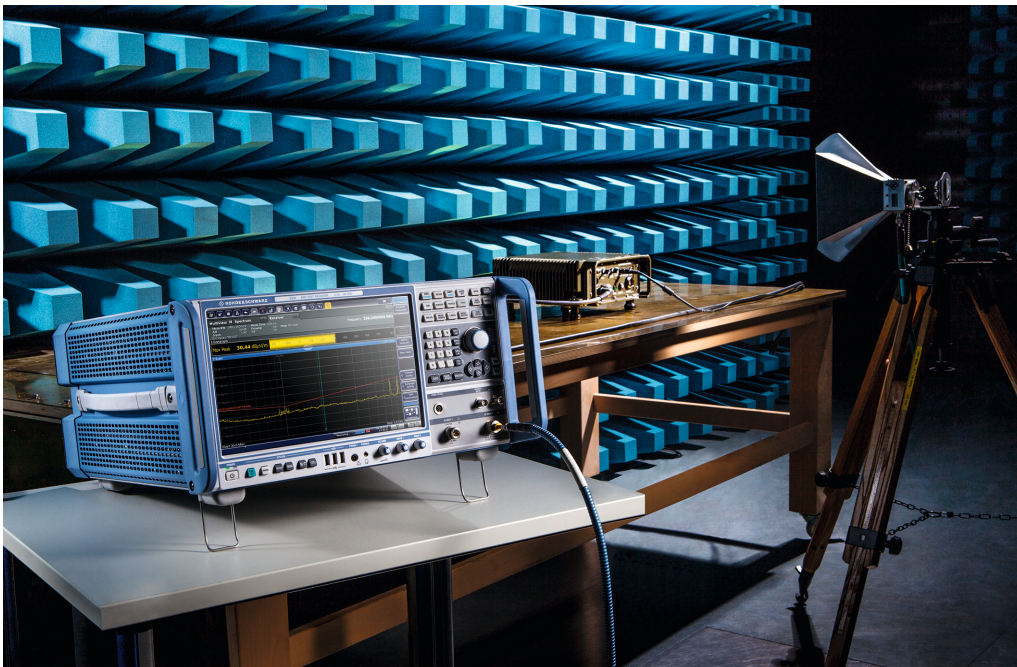
EMI testing in an anechoic chamber.
