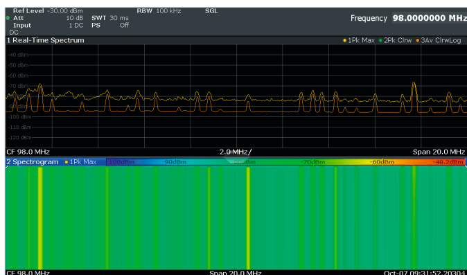
Realtime spectrum with spectrogram.
