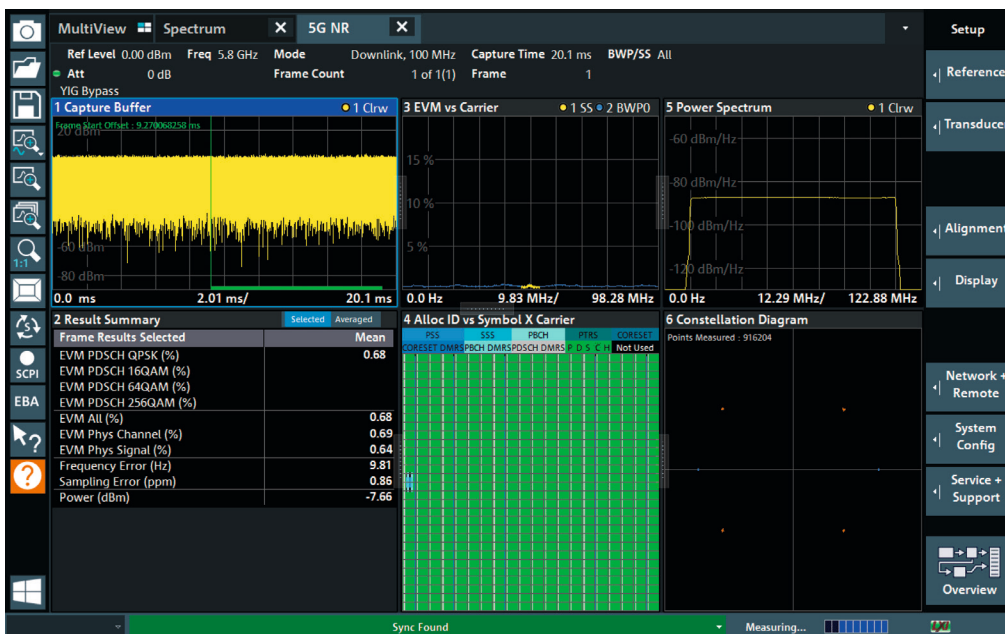
Analysis of a 5G NR signal with the R&S®FSVA3-K144 (downlink) and R&S®FSVA3-K145 (uplink) options
