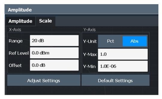
Figure 7-41: Scale settings for CCDF diagram
