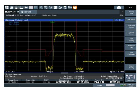
Figure 7-35: Detected peak display in SEM measurement
