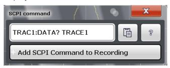
Figure 13-6: SCPI command dialog for a trace in a result display
