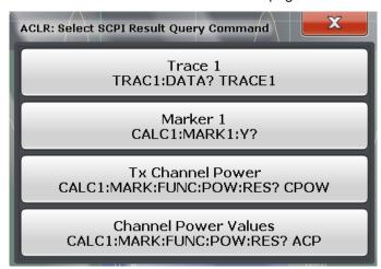
Figure 13-5: Possible result query commands for an ACLR measurement
