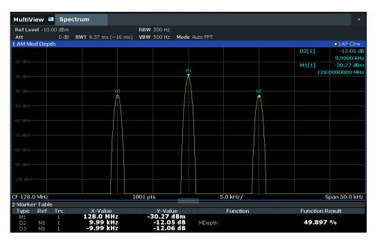
Figure 7-10: Measurement of the AM modulation depth
