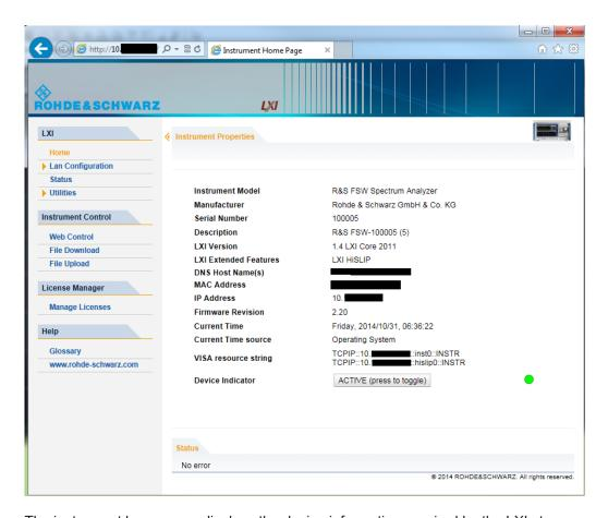
The instrument home page displays the device information required by the LXI standard including the VISA resource string in read-only format.
