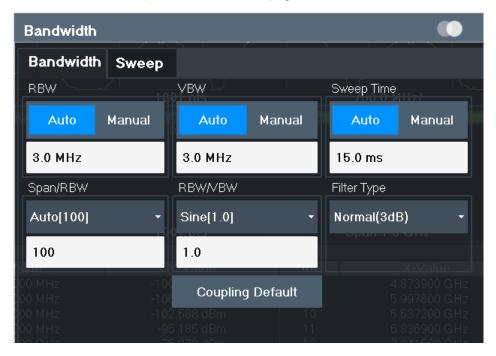
Figure 8-15: Bandwidth dialog box for RF measurements
