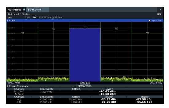
Figure 7-21: Measuring the channel power and adjacent channel power ratio for CDMA2000 signals with zero span (Fast ACLR)
