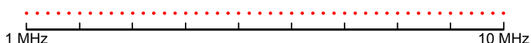
Figure 7-21: Linear x-axis scaling: the distance between the sweep points is equal, e.g. 200 kHz
