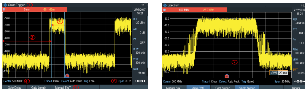
Figure 8-11: Gate trigger measurement
