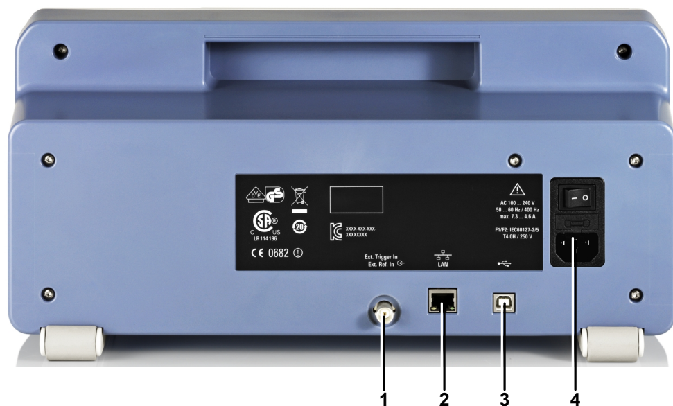
Figure 4-2: Rear panel of the R&S FPC
