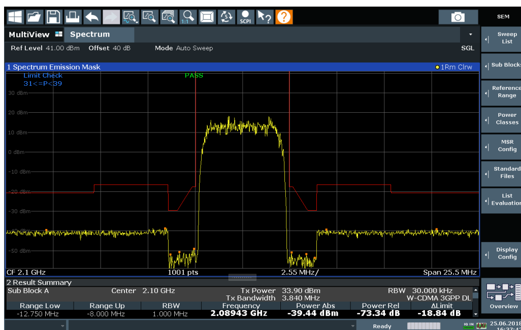
Figure 8-23: Detected peak display in SEM measurement
