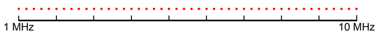
Figure 8-39: Linear x-axis scaling: the distance between the sweep points is equal, e.g. 200 kHz
