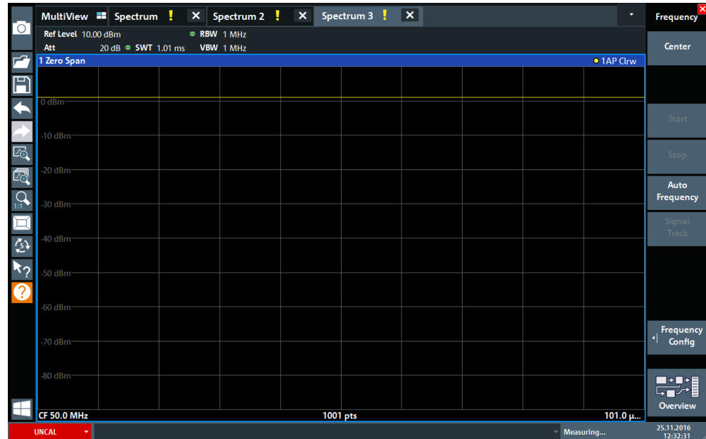
Figure 5-10: Time domain display of the calibration signal
