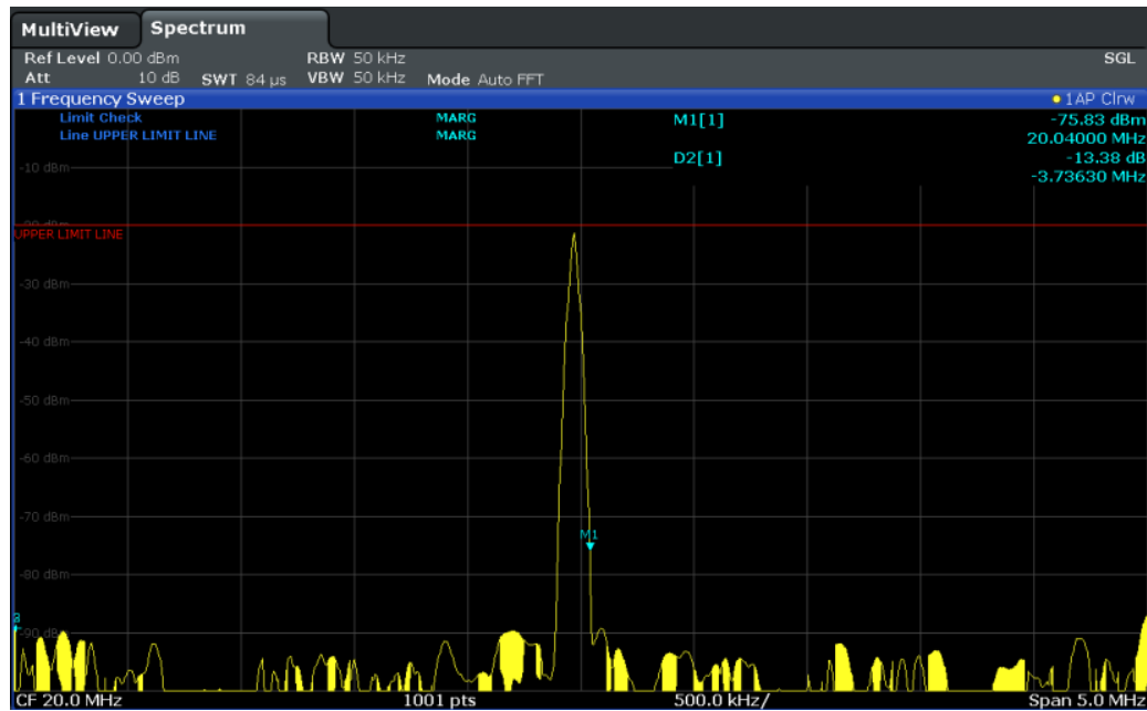
Figure 8-9: Margin violation for limit check
