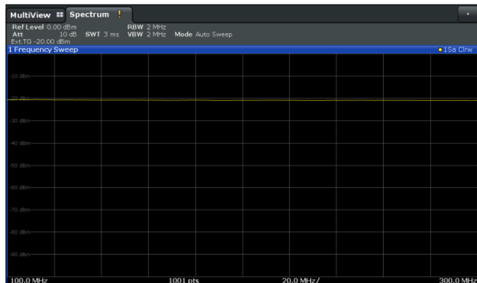
Figure 7-6: Measurement results from generator, analyzer and connecting cables
